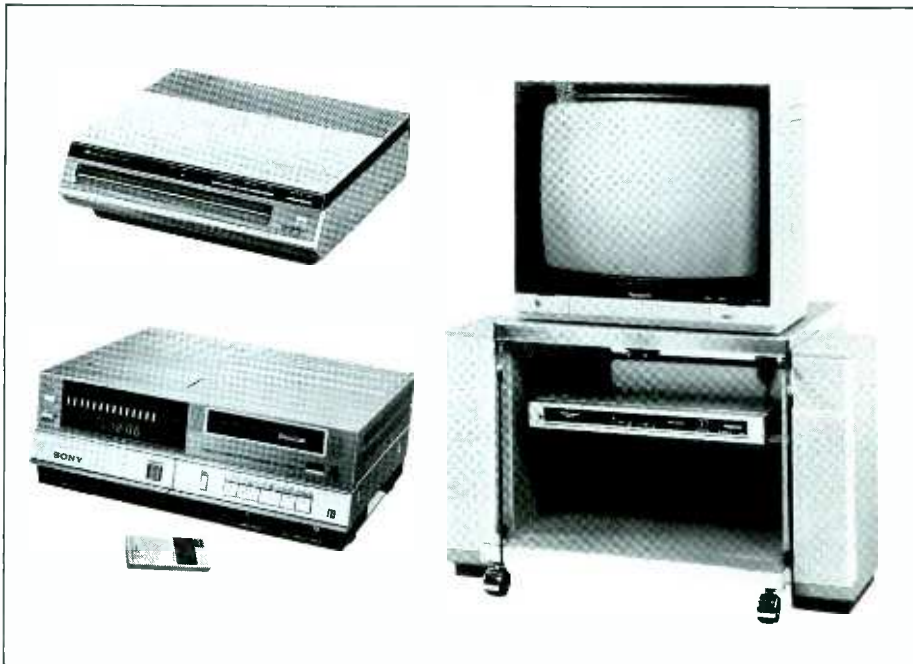
The television set is evolving into a "video component ensemble," with separate monitors, tuners, and speakers (right), allowing components such as video disc players and VCRs (left) to be added on easily.
