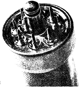
Fig. 5 The base of a key valve, showing the cut-outs for the elevations of the glass base, thereby giving a sufficiently long leakage path between the pins and the screen plate.
