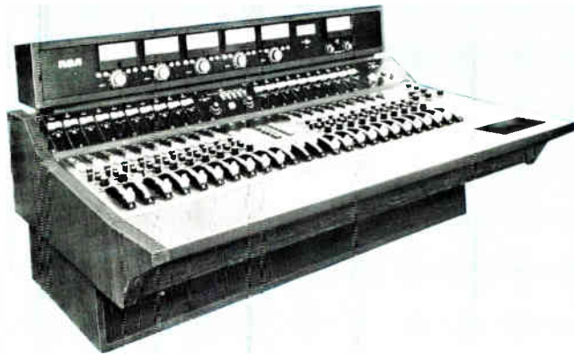
Built especially for Lewron Television in New York City, this is one of two custom audio consoles recently installed. The console offers 20 inputs, which accept either high- or low-level signals, fed to any or all of four output channels. A fifth output channel is equipped with built-in AGC. Each output channel feeds a one-by-two splitter. Also included is a slating switch and a built-in tone oscillator.
