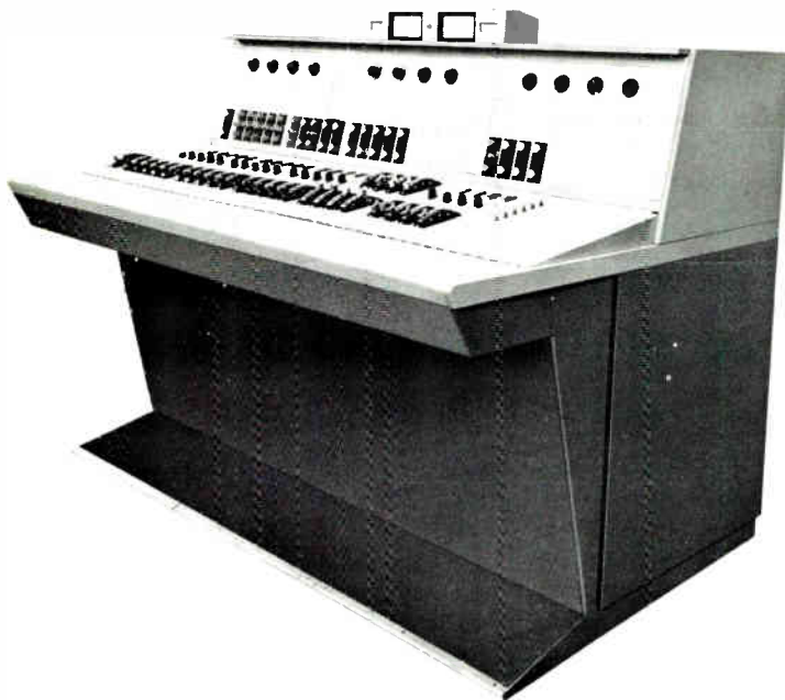
Now serving WLAC's production department, this custom-built console features 45 mike inputs via 15 three-input preamps in addition to one for the announce booth. A pushbutton matrix provides for 24 high-level inputs to the console. The facility includes each send-and-receive, equalization in eight channels, (moveable to any position). The two output channels contain AGC capability, cue, foldback, monitoring and muting.
