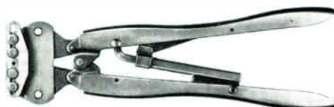
AMP Crimping Tool MI-556674 for BNC Connectors shown right.
