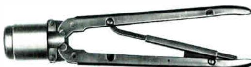
AMP Crimping Tool MI-556671 for UHF Connectors shown right.
