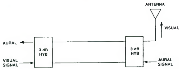
Figure 88. Aural signal applied to back-to-back hybrids.
