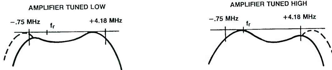
Figure 61. Nonsymmetrical response caused by the amplifiers outside the transmitters bandpass. Solid line is transmitter overall response. Dotted line is the part of PA response outside of the transmitters bandpass.
