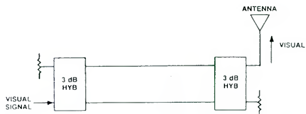
Figure 87B. Visual signal applied to back-to-back hybrids.
