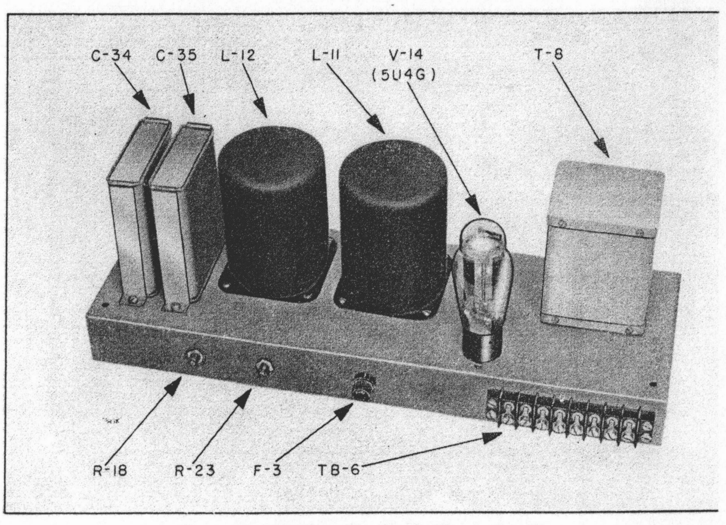
Figure 15. Modulator Bias Supply Chassis: Top View.
