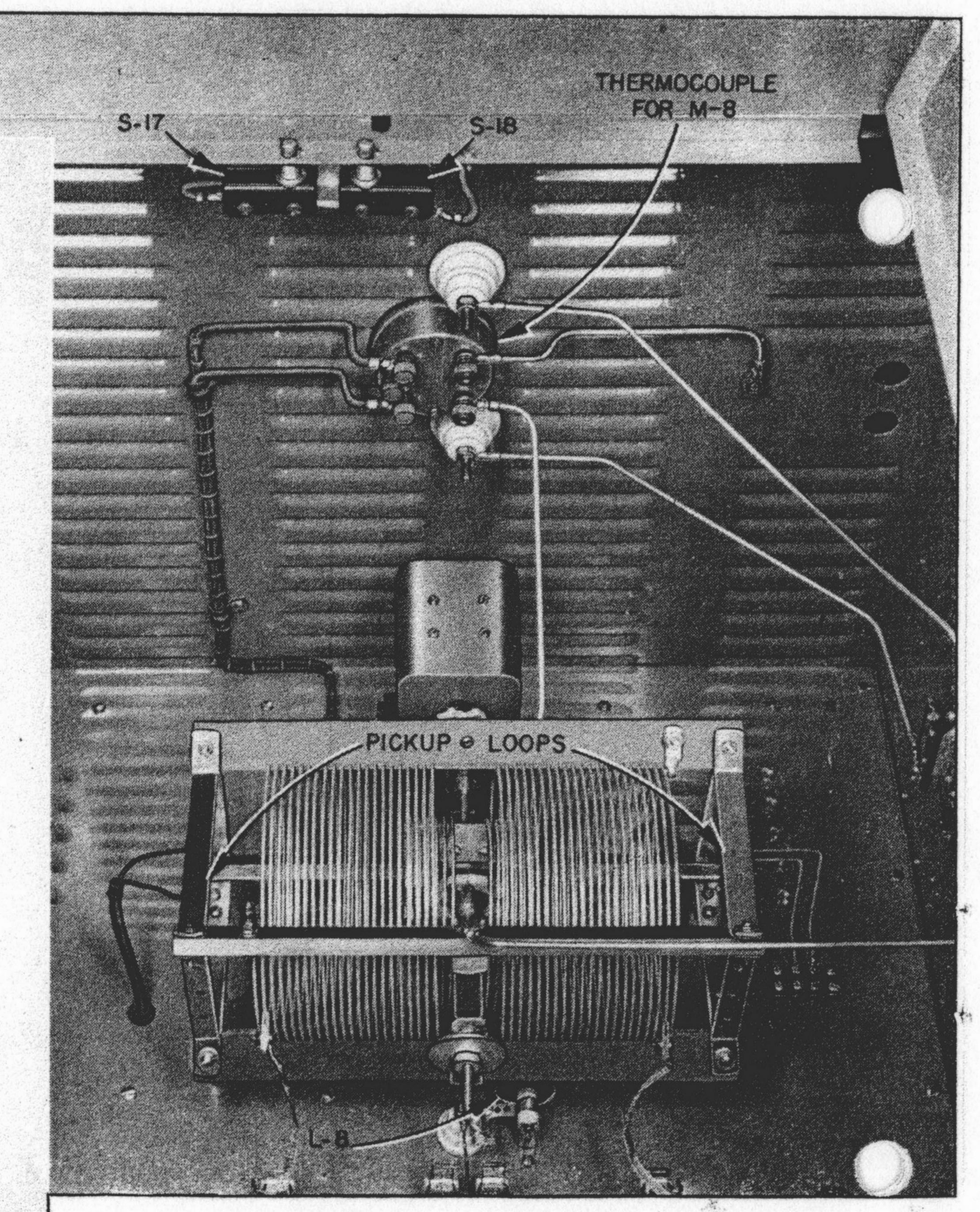
Figure 7. Top Rear View of Transmitter,
