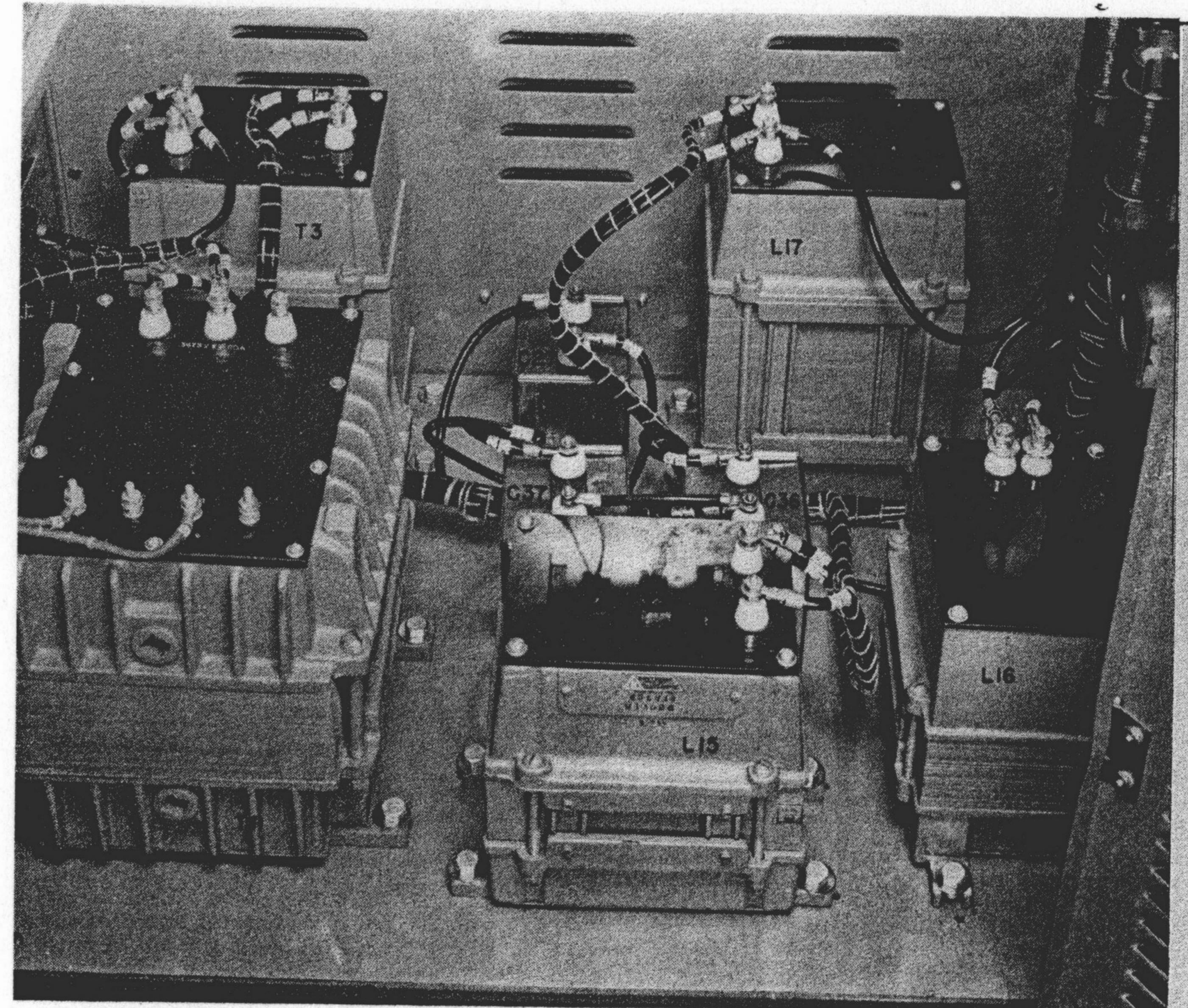
Figure 16. Top Rear View of Transmitter, Showing Lower Components.
