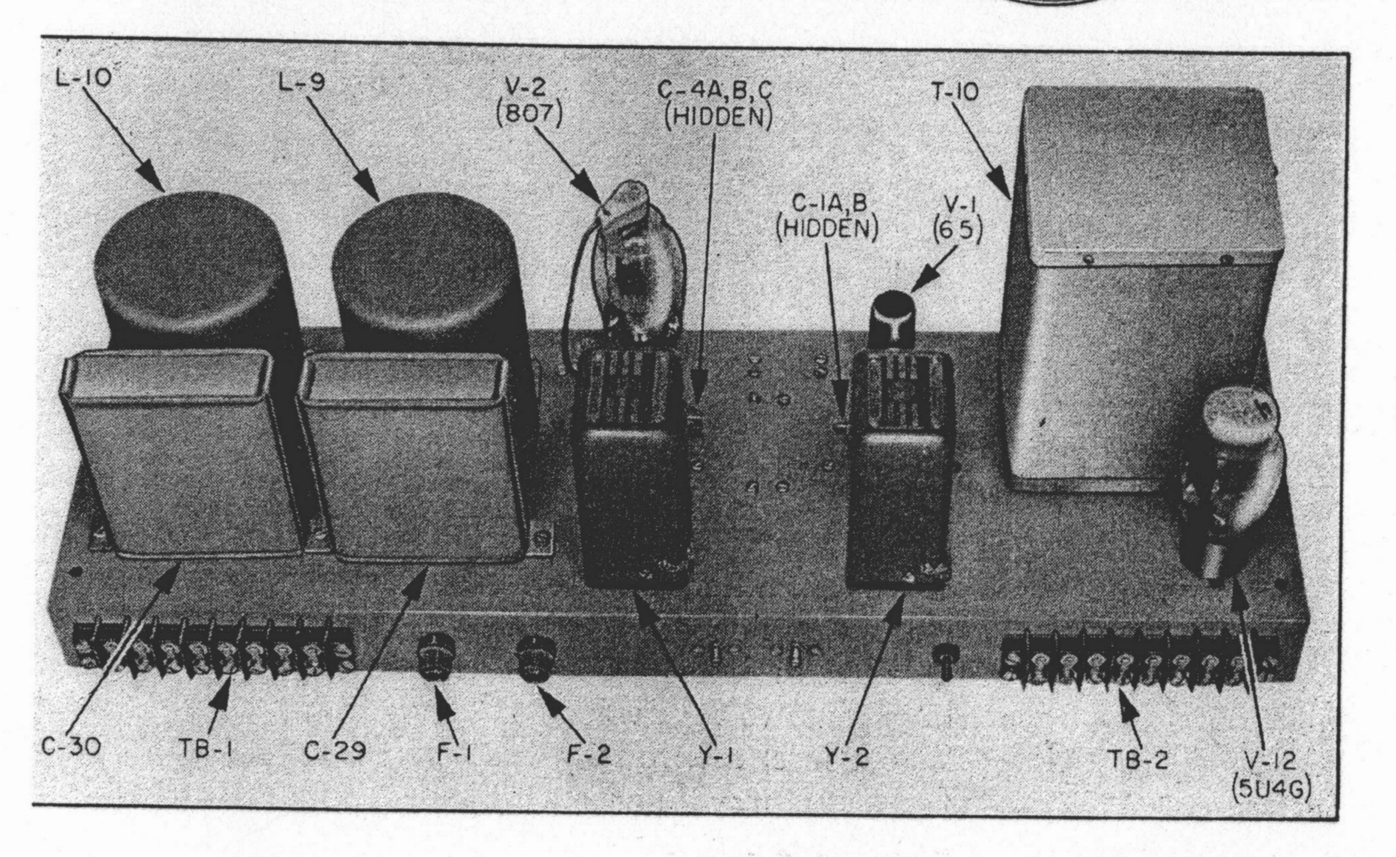
Figure 2. R.F. Exciter: Top Rear View. (C-49 and C-64 are located between Y-1 and Y-2; S-1 to the right of Y-2.)
