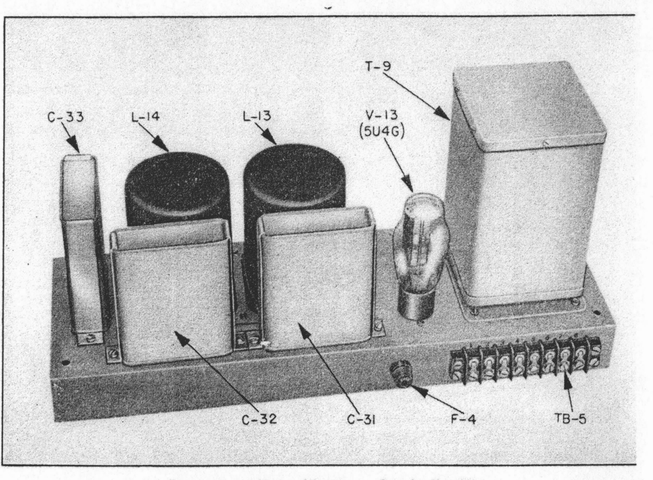
Figure 13. A.F. Amplifier Power Supply: Top View.
