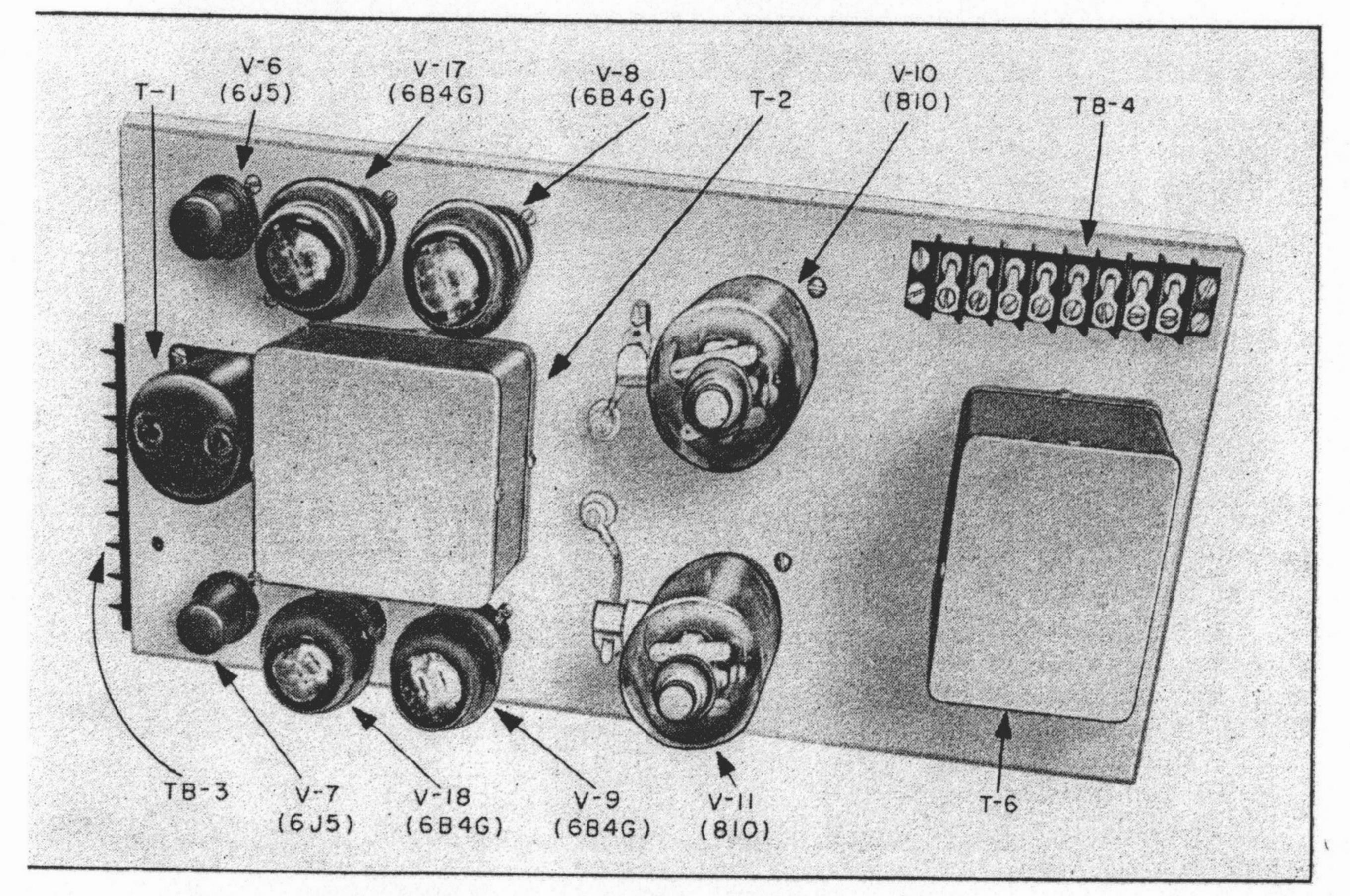
Figure 9. A.F. Amplifier Chassis: Top View.
