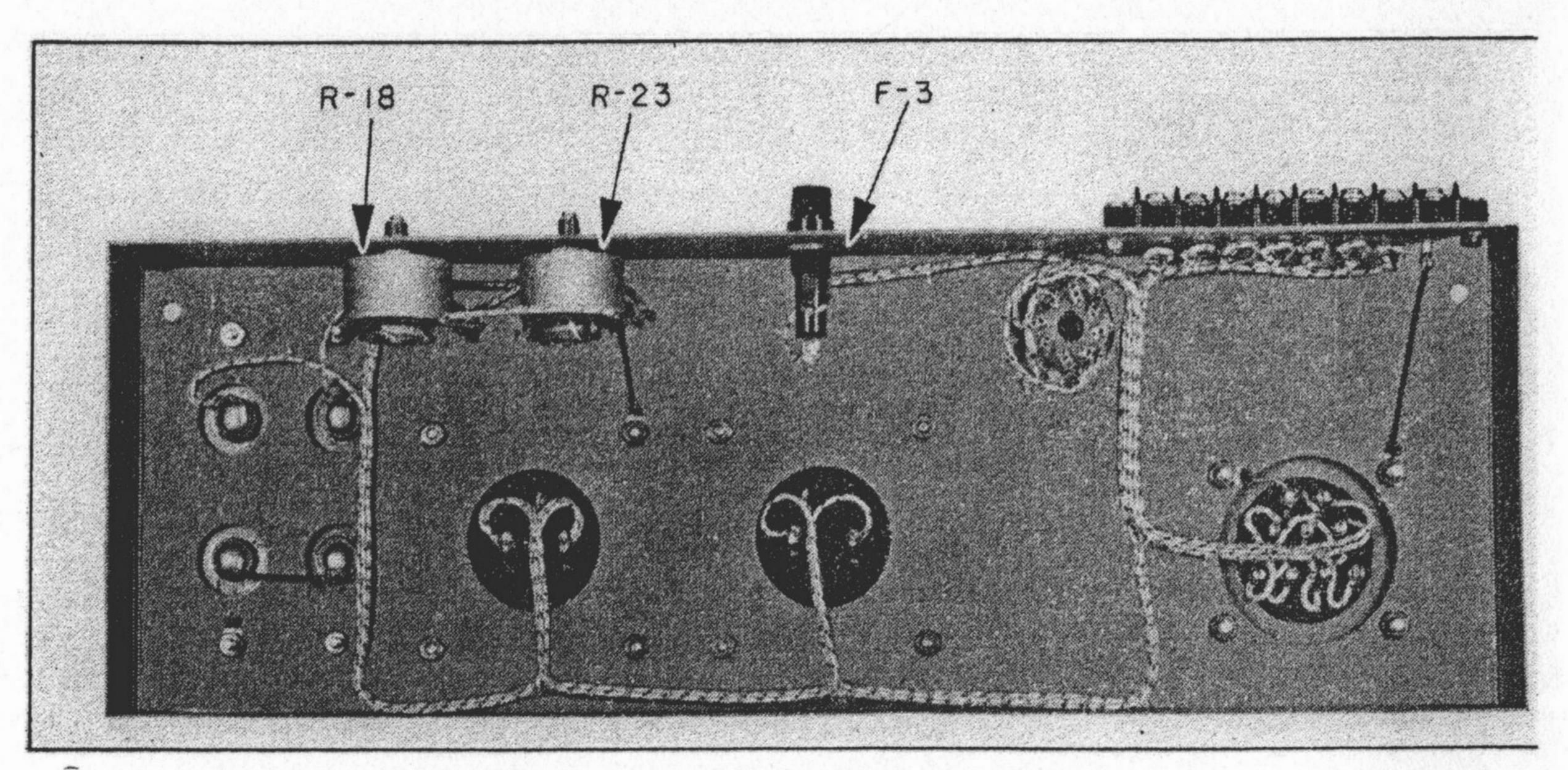
Figure 14. Modulator Bias Supply Chassis: Underside.
