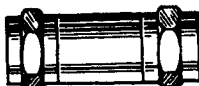
F-71 MALE COUPLING ADAPTER. Mates two F-81, F-1159, F-101-59, F-61 and A-61. $1.60 List
