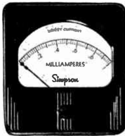
MODELS 27, 37, 47, 57 3 1/2" RECTANGULAR CASE. Width, 3"; height, 3 3/8". Mounts in round hole. Body diameter, 2 3/4". Scale length 2 9/16". Bakelite case.
