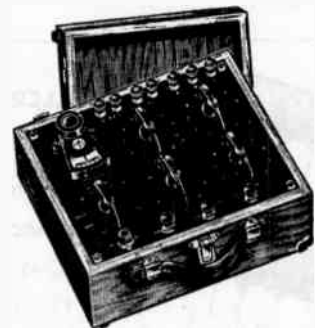
No. 629 FAULT LOCATION BRIDGE
