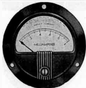
3" ROUND CASE — SHROUD STYLE. Flange diameter, 3 1/2"; depth overall, 2 1/4"; body diameter, 2 3/4"; scale length, 2-9/16". Bakelite case.
