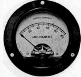
2" ROUND CASE—OPEN FACE STYLE. Flange diameter, 2 3/4"; depth overall, 2 5/8"; body diameter, 2 1/4"; scale length, 1 1/8". Bakelite case.
