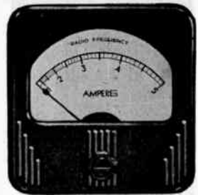
2" RECTANGULAR CASE. 2 3/8" square. Mounts in round hole. Body diameter, 2 3/8". Bakelite case.
