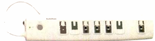
7-outlet appliance surge protector with child-safety outlet covers. 788-joule rating. 15-amp circuit breaker. On/off pushbutton. Power-on light. 20dB noise filter. 7-ft. power cord with right-angle plug. Up to $5,000 Connected Equipment Guarantee #61-2440
