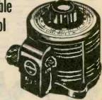
Variable autotransformer of toroidal core design. Ideal for adjusting line voltages and hundreds of other applications in laboratory, workshop, etc. Heavy-duty line cord & plug, on-off switch, AC outlet, fuse. AC input: 110-125 volts at 50/60 Hz. 273-043.
