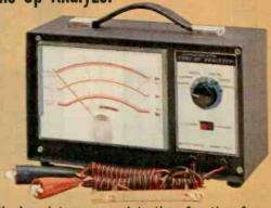
Does every electrically based tune-up and testing function for 4-6-8 cylinder engines. 6" D'Arsonval meter with jewelled movement has color-coded scales. Reads high rpm (0-6000), low rpm (0-1200); 0-16 VDC, 0-80 amps, and cam dwell (0-45° & 0-60°). Rotary function selector, 6' color-coded test leads, external shunt bar with leads. Sturdy metal case with carrying strap. Instructions and charts included. Size, 9%x5%x4%"
