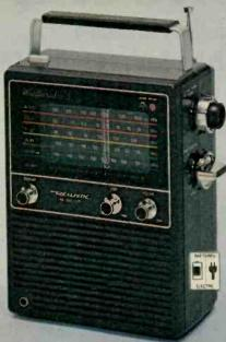
Realistic Weatheradio-5. Press the top-mounted button for National Weather Service reports and forecasts instantly, without retuning! Tune commercial aircraft (108-136 MHz), police, fire and public service (144-174 MHz), worldwide shortwave (6-18 MHz), AM or FM. Fine-tuning for both shortwave and weather, adjustable VHF squelch reduces noise during standby. Variable tone control, 3½" speaker. External antenna jack, ¼" phone jack. With 4 "C" cells, AC cord. 10¾x8¾x3½". 12-755. U. L. listed. 79.95
