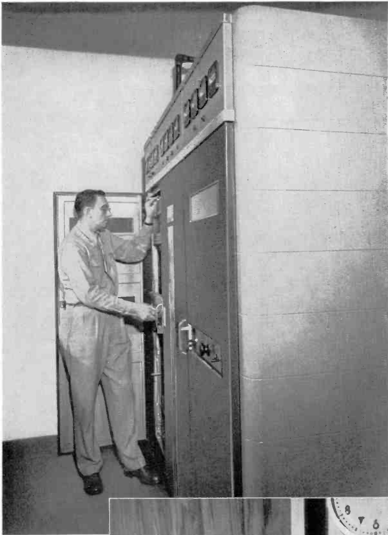
Three kilowatt FM transmitter, Type BTF-3B, as viewed from studio B, at WATG-FM, Ashland, Ohio.
