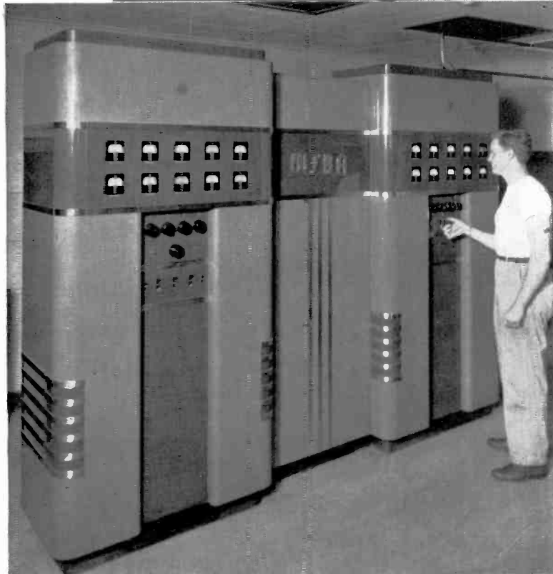
Fifty kilowatt transmitter, Type BTA-50F, with control console and extension cabinets containing phasing equipment, at KMPC, Hollywood, Cal.
