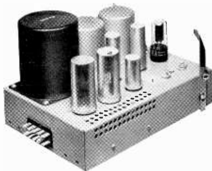
Back view showing multi-contact connection plug
