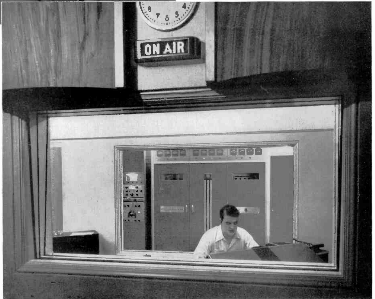
Three kilowatt FM transmitter, Type BTF-3B, as viewed from studio B, at WATG-FM, Ashland, Ohio.
