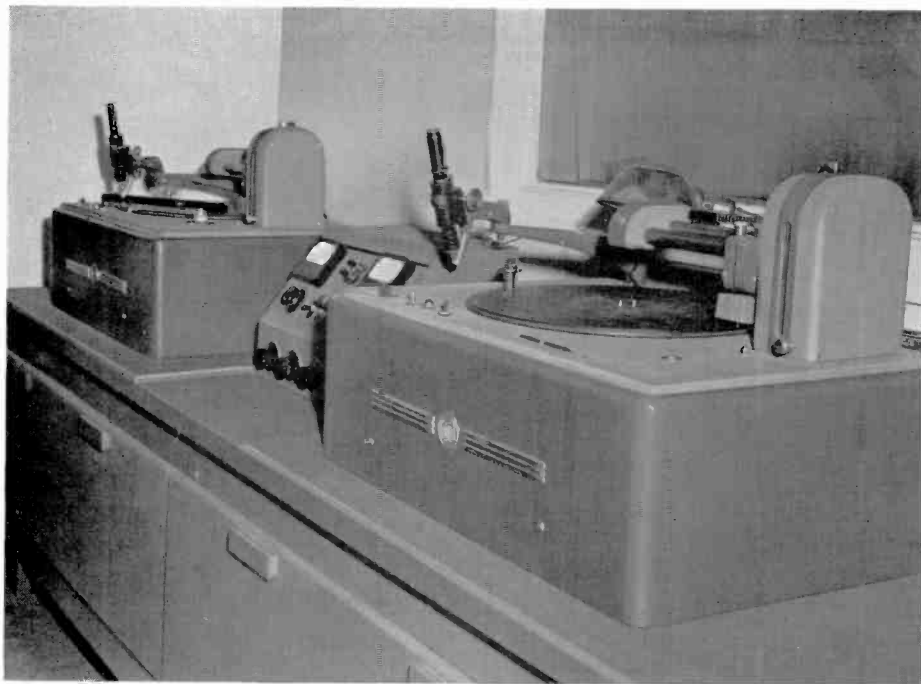
An ideal recording installation at KECA, Los Angeles, Calif., showing two of the four RCA 73-B Professional Recorders. Note the conveniently located overhead lighting, the large size auction duct, and relatively short length of hose for chip removal.
