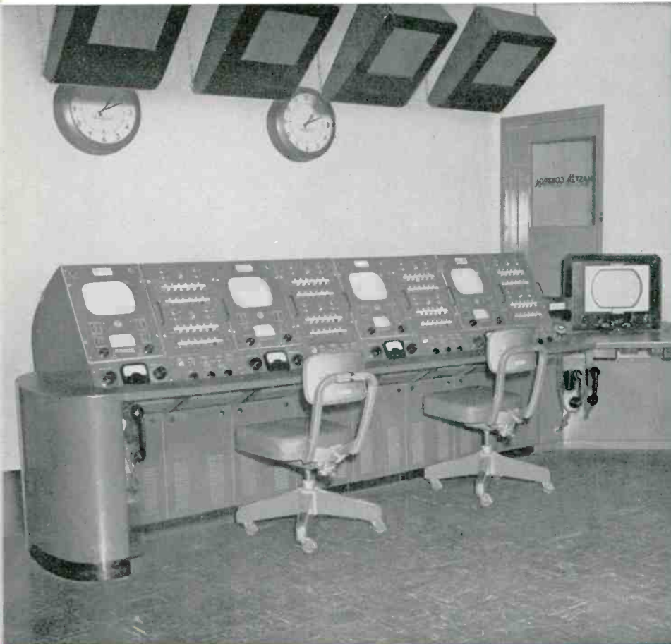
The studio console design shown above employs varied colored knobs and switch handles for easy and quick identification of individual controls. All escutcheons and dial plates are of attractive, long-wearing nickel silver.
