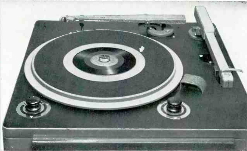
Arrow above points to the MI-11886, 45 RPM Adaptor, mounted on the 70-D Turntable
