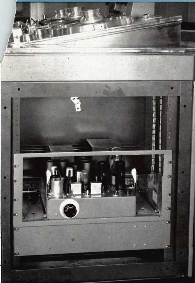
▲ End view of the Editing Machine illustrating how removable end panels make the amplifier easily accessible.
