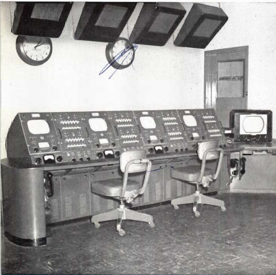
The studio console design shown above employs varied colored knobs and switch handles for easy and quick identification of individual controls. All escutcheons and dial plates are of attractive, long-wearing nickel silver.
