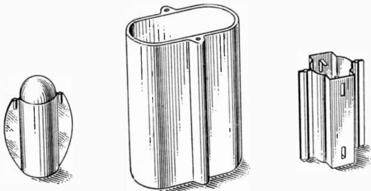
Typical Anode Structures
