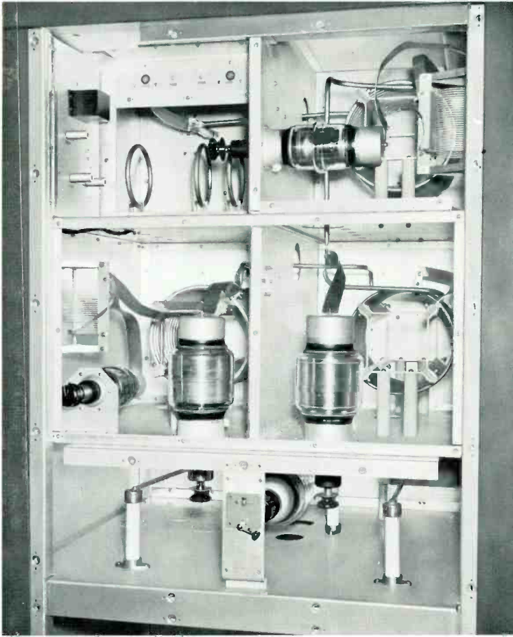
Upper rear of exciter portion of the BTA-50J showing the combining and output networks.
