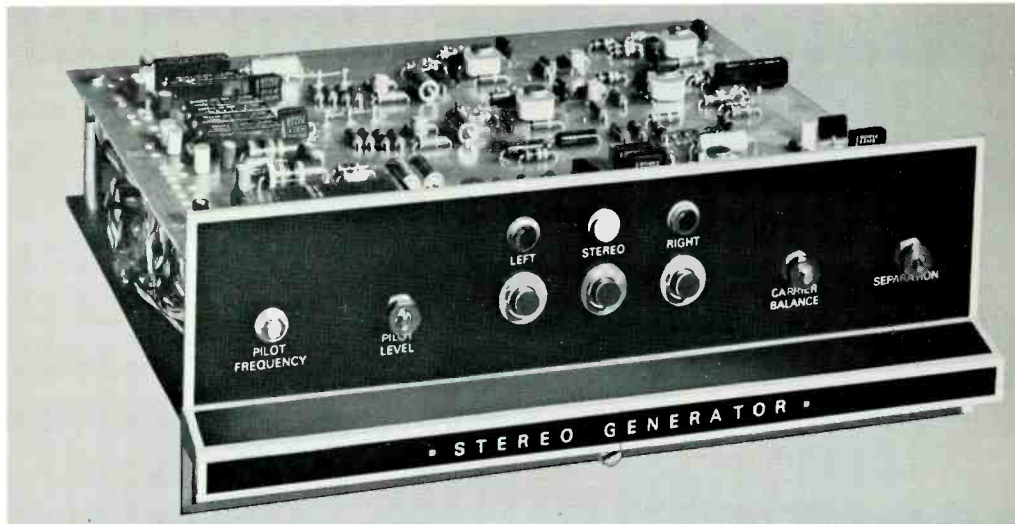
BTS-1B Stereo Generator.
