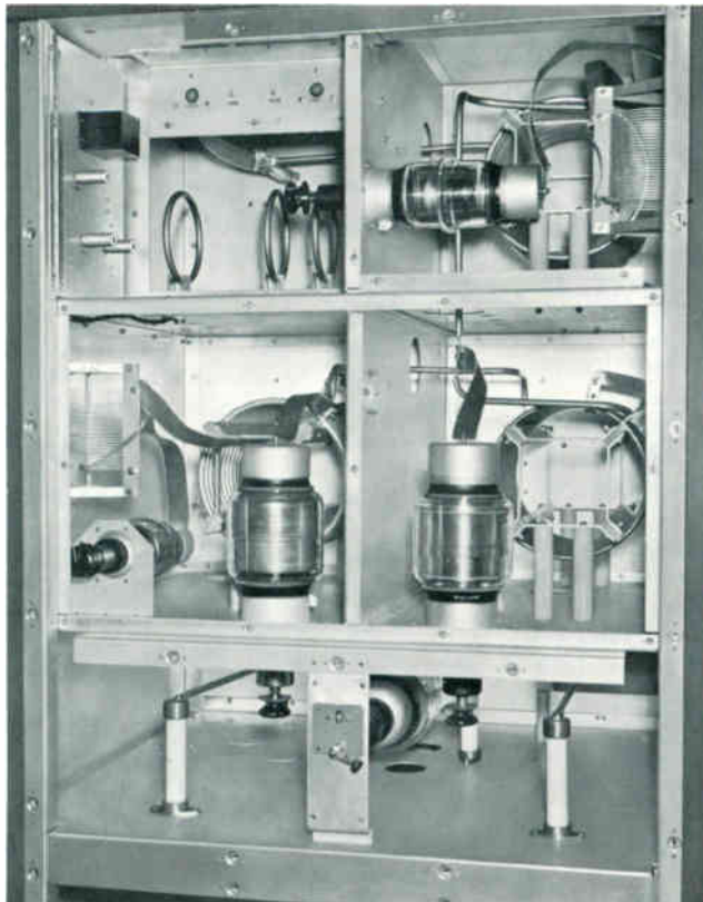
Upper rear of exciter portion of the BTA-50H1 showing the combining and output networks.
