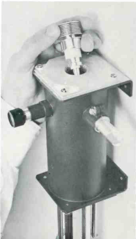
CERAMIC-TETRODE DRIVER AMPLIFIERS couple exciter/modulator output to the klystrons. The drivers are identical for aural and visual portions thus allowing interchangeability.
