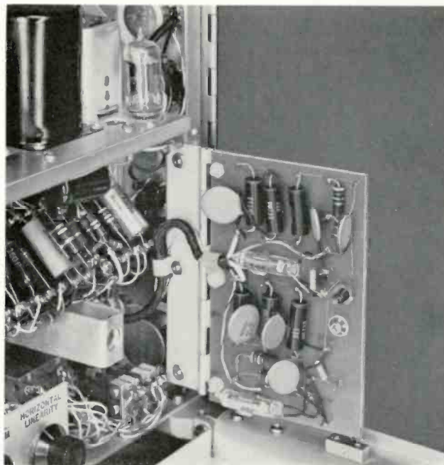
TK-14 high voltage regulation circuit utilizing gas discharge tube provides improved image orthicon stability.
