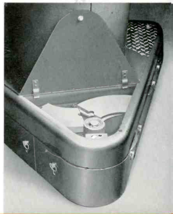
◀ Pedestal with housing removed, showing placement of lead weights for counterbalancing camera.
