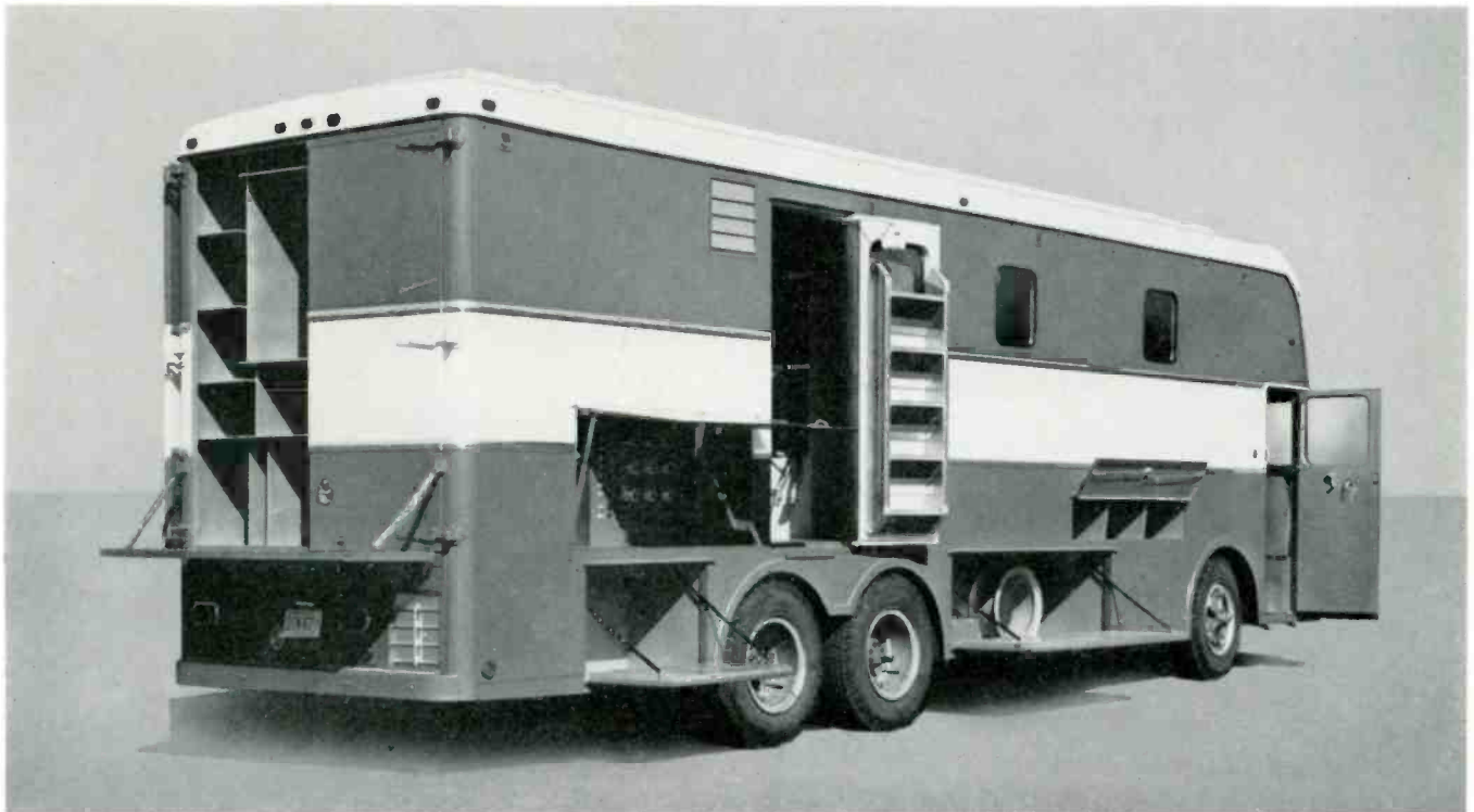
An RCA custom bus design illustrating maximum utilization of all available space for equipment storage.
