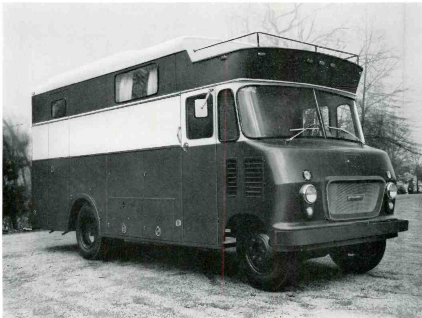
TJ-70D Mobile Camera Production Unit showing distinctive step in forward roof line, fiberglass front end, and deluxe trim. Reinforced roof affords vantage point for use of field camera chain.
