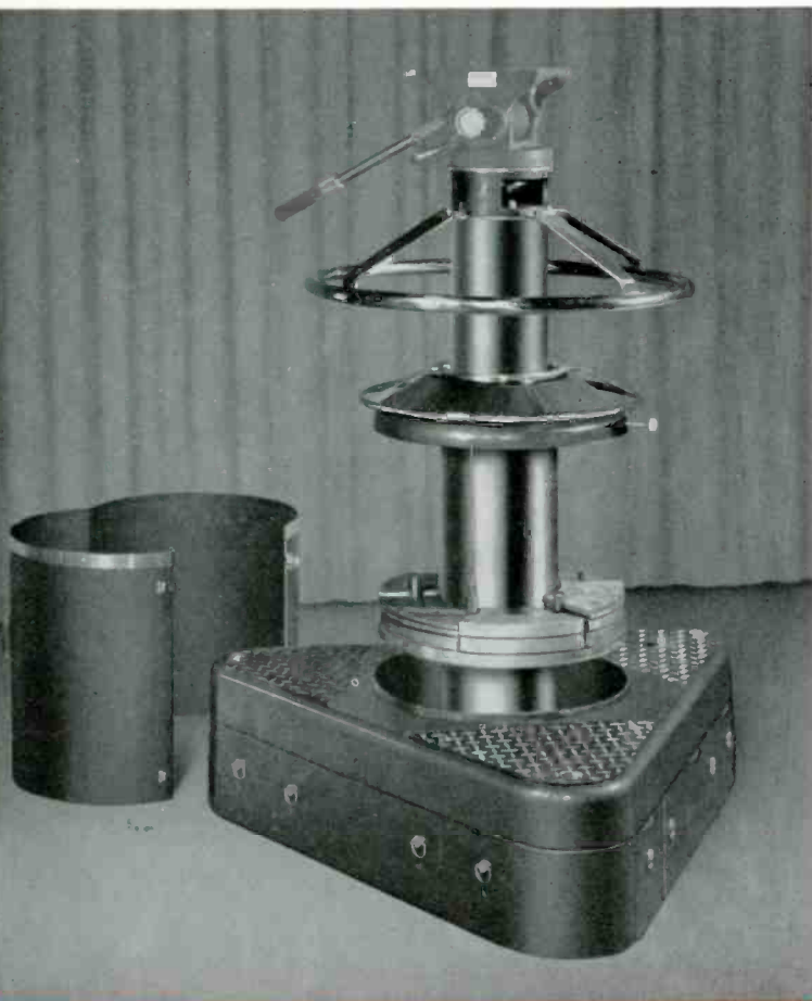
◀ Pedestal with housing removed, showing placement of lead weights for counterbalancing camera.
