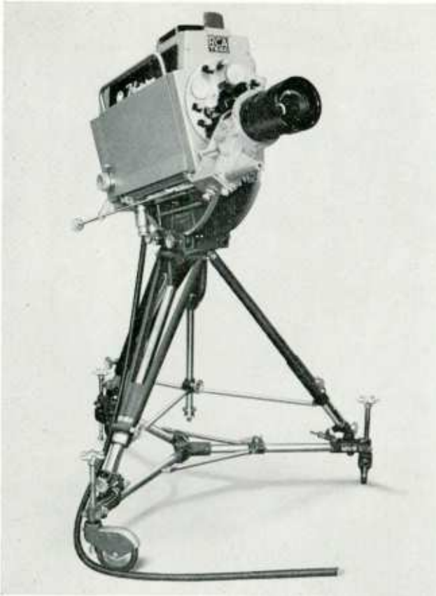
The Model 10-2-1-B Angenieux Zoomar Lens shown mounted directly to turret of RCA TK-60A I.O. Camera. Control rod governs both zoom and focus of these versatile lenses.
