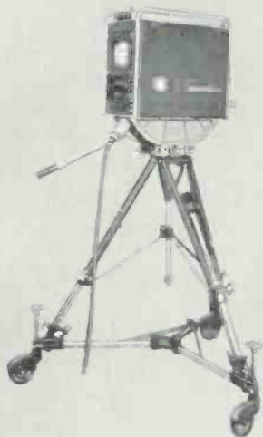
BASIC CAMERA CHAIN WITH LOCAL CAMERA CONTROLS
