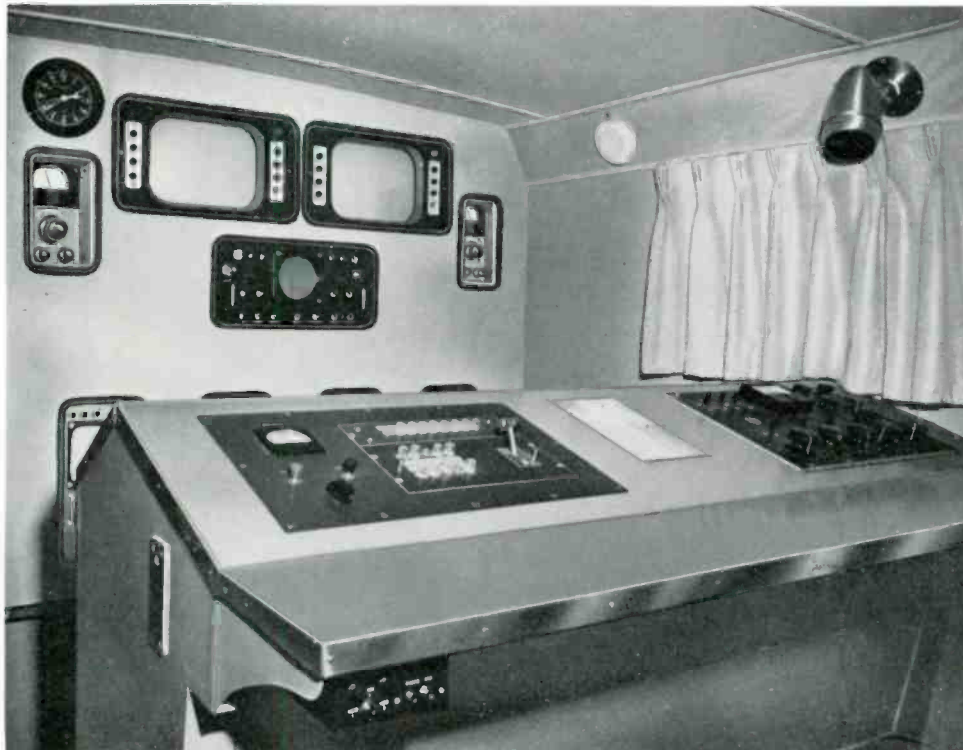
Interior view of the TJ-70D showing switching console overlooking the equipment frame and video position in the operating compartment.
