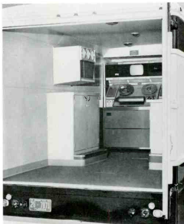
TJ-72 interior as viewed through rear doors. Note Type TR-22 Television Tape Equipment with air conditioner and storage cabinet at left.
