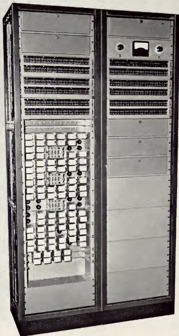
Master control audio relay switching system recently installed at Station KSTP. Shown at right is compact control panel designed to fit a standard 22-inch console housing. Three VU meters for line, program and preview, monitor controls, pushbutton controls for preview and program busses and selectable auxiliary fader inputs are shown among other facilities. To the left are rack-mounted facilities including amplifier shelves, jack fields, and relay switcher.
