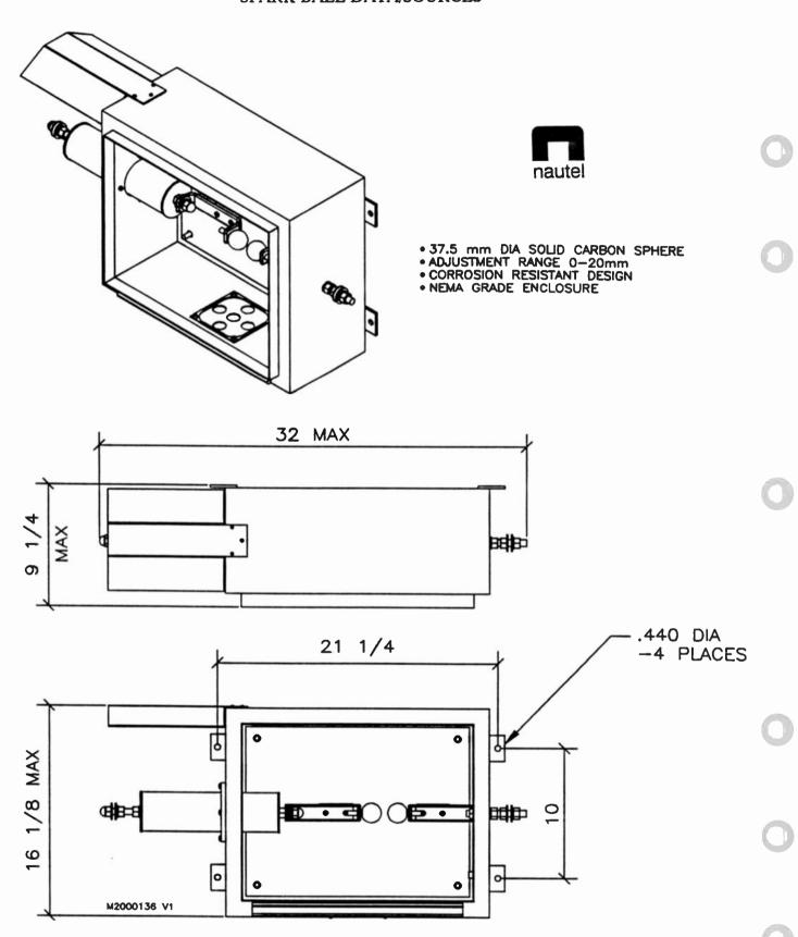
Figure C-2 NAX185 Enclosed High Voltage Spark Gap
