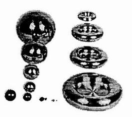
rent spark gaps or for terminations. Diameters of the standard spheres range from 2.5 cm to 50 cm (.98 in to 19.68 in). The non-melting carbon spheres are used for calibrated spark gaps, lightning arresters on antennas, power supply overvoltage, and other transient suppression and high current spark discharge in pulse forming networks. The solid earbon sphere diameters vary from 1 cm to 30.48 cm (.396 in to 12 in).
