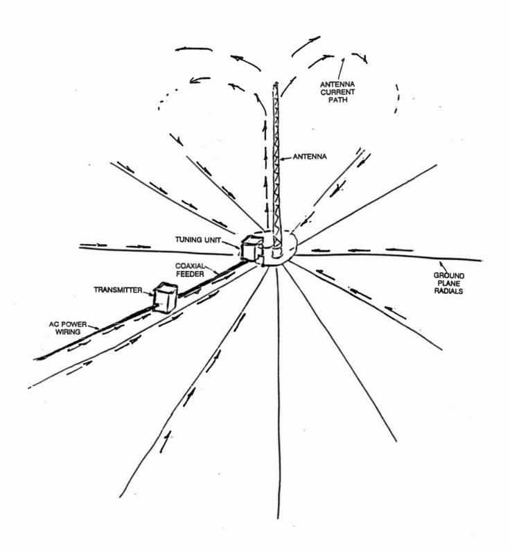
Figure F-2 Antenna Current Feedback
