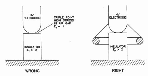
Figure E-1 Stress Control at Electrode/Insulator Interface
