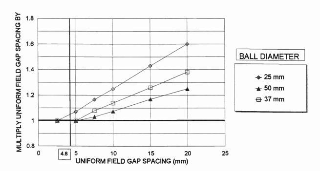
EXAMPLE: Established Uniform Field Gap Spacing = 4.8 mm
