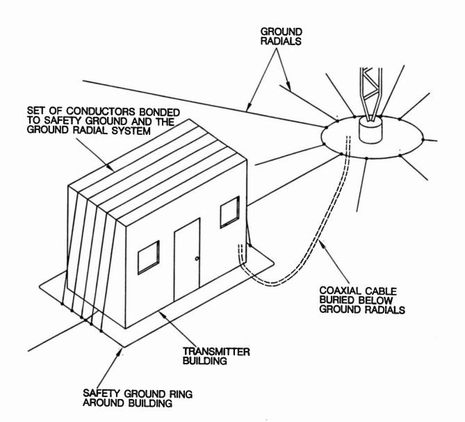
Figure F-3 Screening of Transmitter Building
