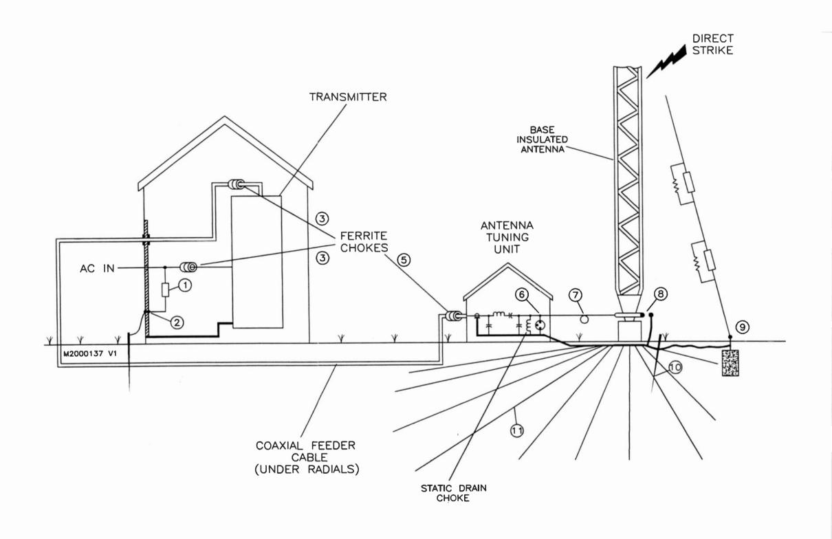
Figure 8 Recommended Installation Configuration
