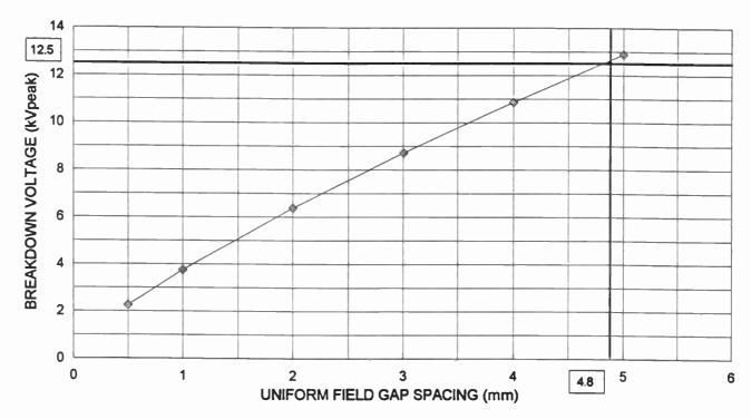
**EXAMPLE:** Established Peak Voltage = 12.5 kV<sub>PEAK</sub>
