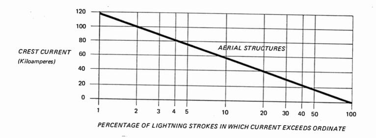
Figure 3 Magnitude Distribution of Currents in Lightning Strokes to Structures
