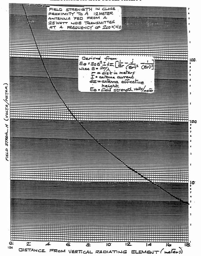
Figure F-1 Electromagnetic Feedback
