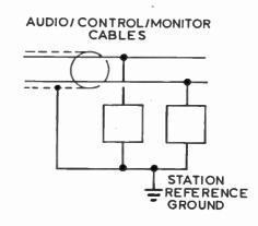
Figure 4 Surge Protector Connection on Power, Audio, Control and Monitor Wires
