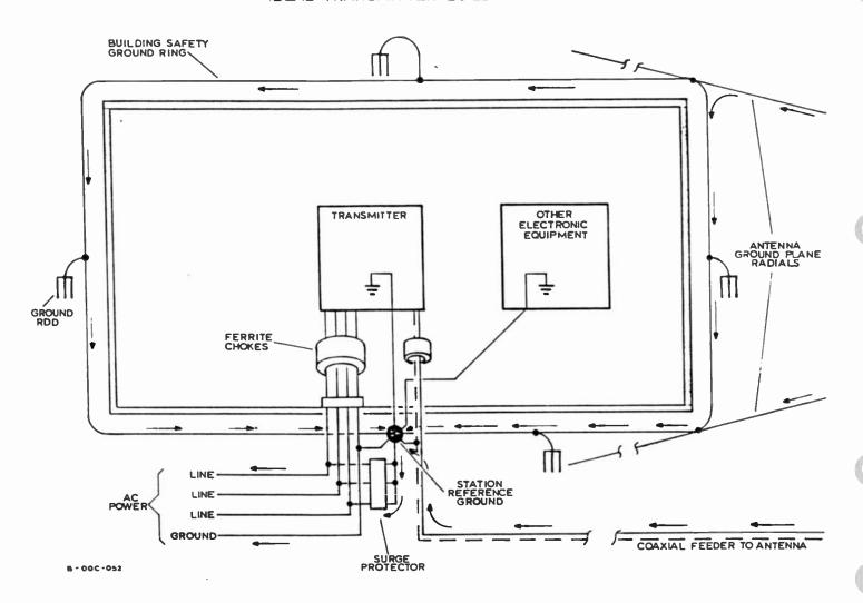
Figure D-2 Ideal Transmitter Building Layout (Electrical Representation)
