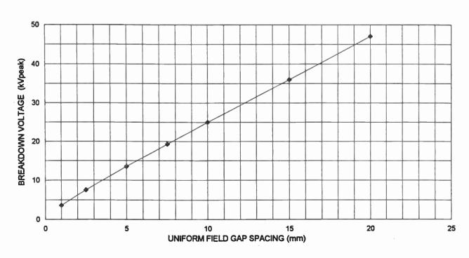
Figure B-3 Determination of Uniform Field Gap Spacing (High Volts - Up to 50 kV<sub>PEAK</sub>)
