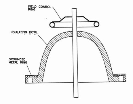
Figure E-2 Typical Feed-Through Bowl Insulator
