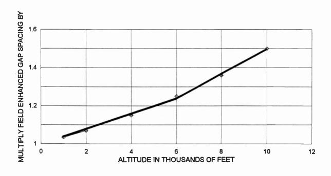
Figure B-6 Altitude Correction Factor
