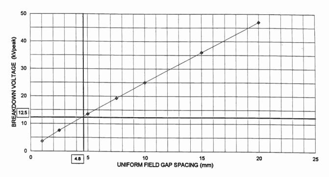
**EXAMPLE:** Established Peak Voltage = 12.5 kV<sub>PEAK</sub>
