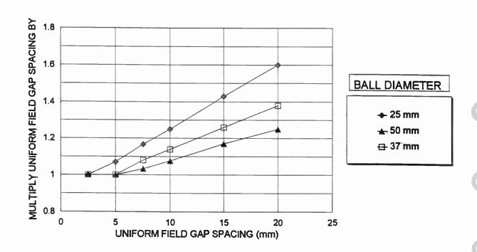
Figure B-5 Spark Ball Diameter Correction Factor
