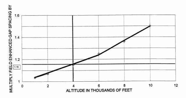
**EXAMPLE:** Site Altitude = 4000 Feet Calculated Altitude Correction Factor = 1.15
