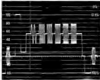
Fig 2. 50% Amplitude Multiburst for use where 100% tests are invalidated by non-linear distortions; e.g., transmitters.
