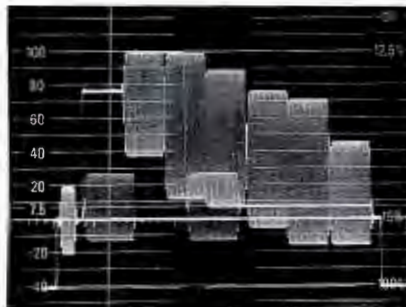
Fig 3. Standard EIA Color Bar Signal defined in RS-189. Setup can be conveniently changed to 10% or 0.
