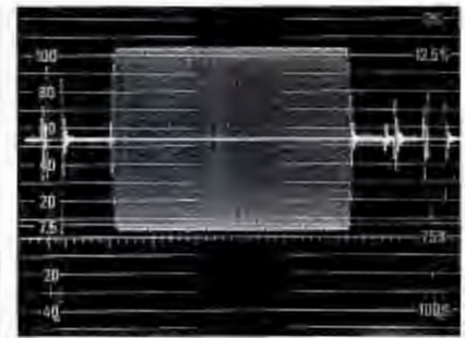
Fig 20. Differential gain measurement on waveform monitor using 10-step staircase. Note absence of luminance transients.
