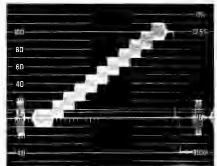
Fig 6. Linearity Test Signal 10 step with 20 IRE subcarrier at burst phase.
