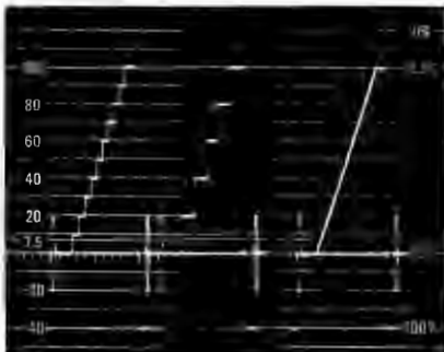
Fig 10. Triple exposure of linearity signals 5 step, 10 step and ramp.
