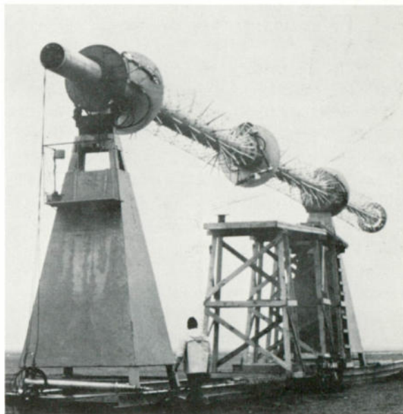
Long view of a three-section Cefec Spiral antenna on test stand on the Sacramento Valley range.
