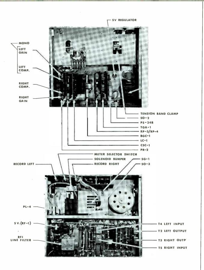
Figure 5-10 790-792 Record Center Top & Bottom Assembled Views
