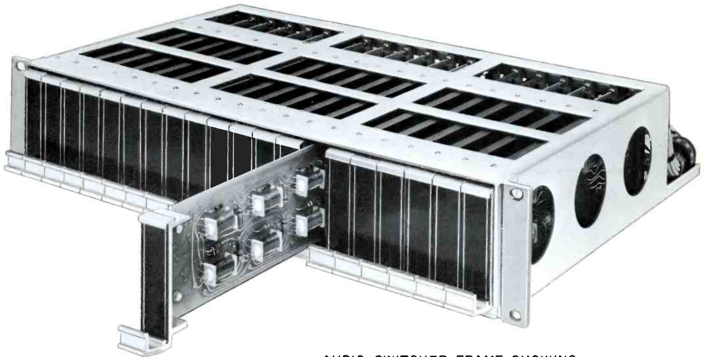
AUDIO SWITCHER FRAME SHOWING SM 8 REED RELAY MODULE
