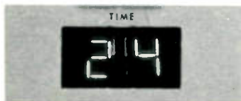
Digital clock, built in, provides the time base. Minutes only are shown. This clock provides all readying pulses for the system.
