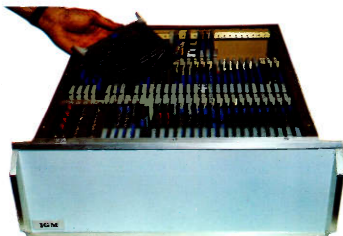
Compact, solid-state plug-in printed circuit modules, above, permit all interfacing required by the basic IGM 630 system to be contained in a single roll-out.
