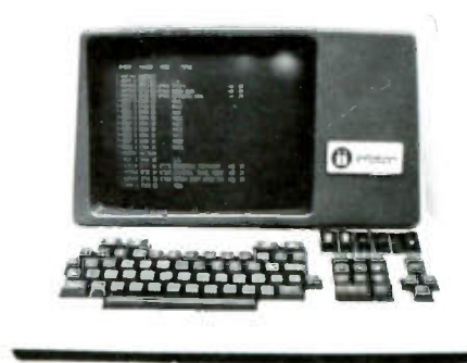
The 24-line CRT keyboard/display unit is standard on the 750 and 770. It allows an operator to correct, add, or delete lines of information at will.
