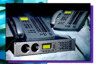
The TWOx12 digital talk show system plugs right into ISDN BRI phone lines. Your callers sound louder and cleaner with the isolation performance that only a true four-wire system can deliver. And if you don't have ISDN in your studio yet, the TWOx12 lets you start with POTS and upgrade to ISDN whenever you're ready.
