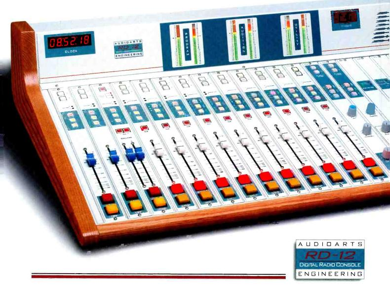
**INTRODUCING THE LATEST RADIO CONSOLE FROM AUDIOARTS:** three stereo outs, two caller superphone module, full-feature control room and studio modules, three VUs, clock, timer, optional intercom, preselect, tape remote panels—and it's **DIGITAL.** That's right, both digital <u>and</u> analog inputs and outputs! INTERESTED? GET IN TOUCH — with AUDIOARTS!
