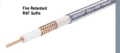
**Barrier Tape**. RNT suffix cables include a double mica barrier tape under the jacketing. This gives additional protection over the RNT1 suffix type cables. The tape is an inert material that does not burn or melt. In the event of a fire, the tape prevents molten dielectric material from flowing out of the slots and igniting.
