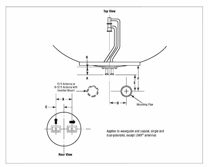
The dimensions presented below are for use in planning transmission line routing for waveguide, coaxial, single-polarized and dual-polarized feeds.
