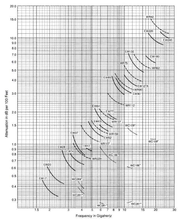
Attenuation curves based on: VSWR 1.0 Ambient Temperature 24° C (75° F) High Conductivity Copper
