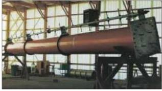
GUIDELINER antenna for WTIU channel 30 undergoing inspection.
