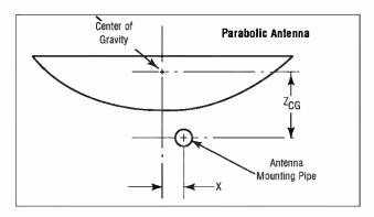
For parabolic antennas, the center of gravity is referenced to the centerline of the antenna mounting pipe as illustrated. Dimension X, the transverse offset, can be found on pages 100 to 110. Dimension  $Z_{\text{CG}}$  and antenna weights with and without ice are tabulated below.
