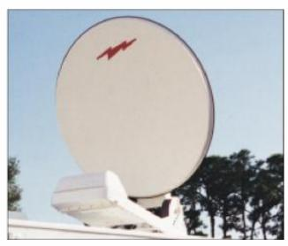
2.4-Meter Transportable SNG Antenna
