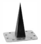
Standard Termination Loads for unused rectangular waveguide port of dual polarized microwave antennas. Maximum VSWR is 1.10. Low VSWR loads for use with circular waveguide transitions are listed on page 223. Flange blanking plates, and termination loads used with IEC flange types are available on request.
