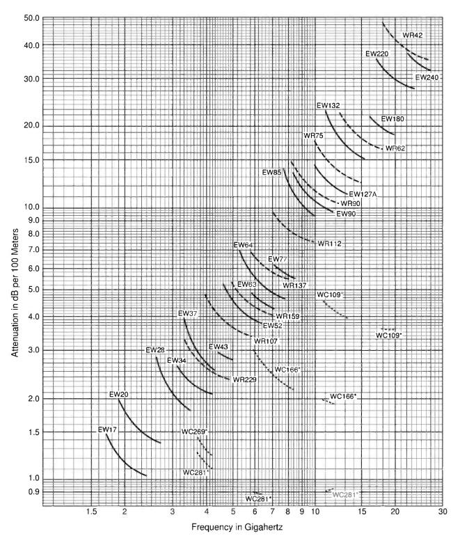
Attenuation curves based on: VSWR 1.0 Ambient Temperature 24° C (75° F) High Conductivity Copper
