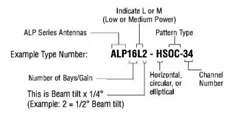
The example antenna is a low power version of a 16 bay, horizontally polarized, omnidirectional antenna, with a beam tilt of 1/2°, for channel 34.
