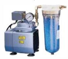
Manual regenerative dehydrators provide an economical automatic drying system. "Automatic" for the 40525A is defined as automatically responding to the pressure requirements of the system, not automatic regeneration of the desiccant. The color indicating desiccant is easily viewed through the canister attached to the unit, providing for programmed replacement. You can replace the desiccant with new desiccant or you can regenerate it.
