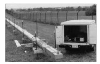
VSWR is 1.08 or better over the channel. Optimization to 1.05 or better at visual carrier is usually possible. And, GUIDELine waveguide does not exhibit band reject spikes associated with coaxial and rectangular waveguide transmission lines because of the extremely small mismatch of the circular flange junction.
