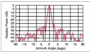
Typical Low Beam Azimuth Pattern at 2.8 GHz
