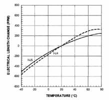
Figure 6 – Electrical Length Change vs. Temperature HJ4-50, HJ5-50
