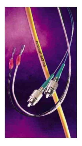
Andrew indoor composite cables combine two Andrew Microcable™ elements with two insulated copper conductors to provide electrical current and fiber optic capability in one cable. This riser rated cable is ideally suited to indoor antenna remoting for cellular and PCS systems and for communication and sensor systems in industrial environments.
