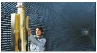
Full Size antenna section undergoing azimuth pattern test in one of two Andrew anechoic chambers dedicated to broadcast products.
