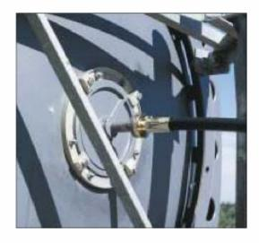
Cables and fitted connectors are available for any standard U.S., Canadian, or CCIR frequency band. Other frequency bands are available on special order. All cable assemblies are sweep tested at the factory to ensure low VSWR performance across the specified operating band.
