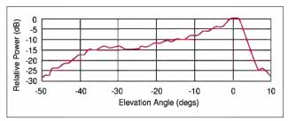
Typical Low Beam Elevation Pattern at 2.8 GHz
