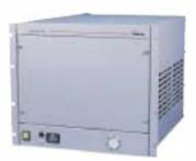
The MT-1700 series automatic membrane dehydrators are the largest rack-mountable units offered by Andrew. They are equipped with the unique Andrew uni-mount system allowing for rack, or free-standing mounting without additional parts. They are designed to supply dry air at a dewpoint of -45°C (-50°F), or better, under the ambient conditions of 95% RH at 49°C (120°F).
