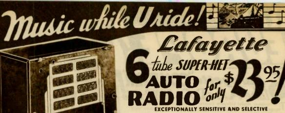
Six tuned circuits (not including the oscillatar tuning) make this ane of the most selective auto radio sets ever built. And through the use of high gain coils in the RF and IF stages together with the new high gain tubes a remarkable degree of sensitivity has been obtained. This assures satisfactory reception on practically any type of auto aerial in use to-day.
