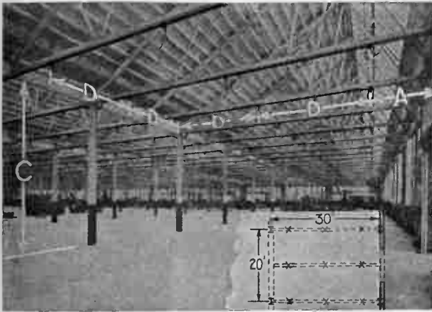
Layout of Outlets for Large Industrial Building
