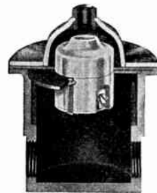
Sectional View of No. 477 Showing Receptacle Mounted on Steel Ring
