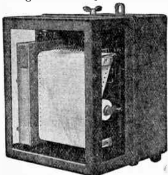
Time Recorder which Makes a Record of Every Call and Time Taken to Answer
