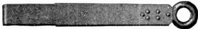
Drop-forged Link Connects Trailer to Pintle Hook. This Is Attached to Drawbar with Automatic Lock Pin
