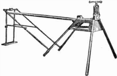
Large Size, with Hinged Pipe Vise and Rear Support
