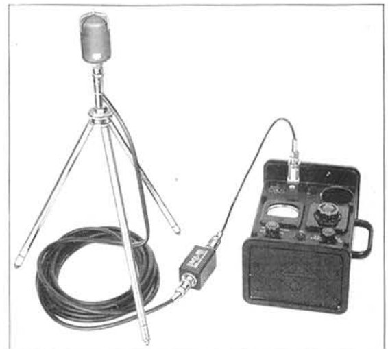
(B) Microphone and transformer plug into the sound-level meter as shown above.
