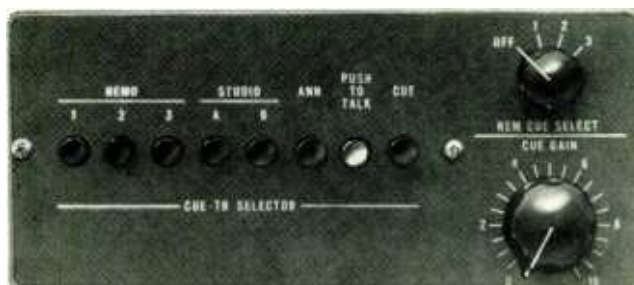
Cue/talkback selector and gain control panel
