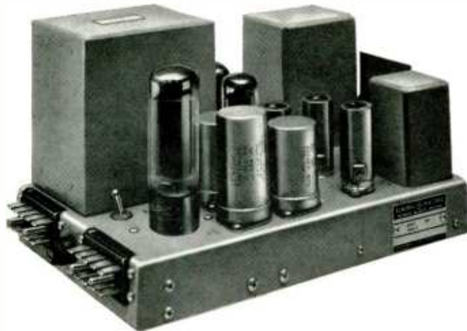
Rear view of amplifier Type BA-14-A showing plug-in construction
