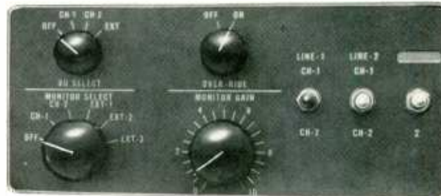
Monitor, VU meter and line output control panel
