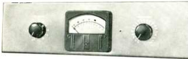
Program level indicator panel, Type FA-1-A
