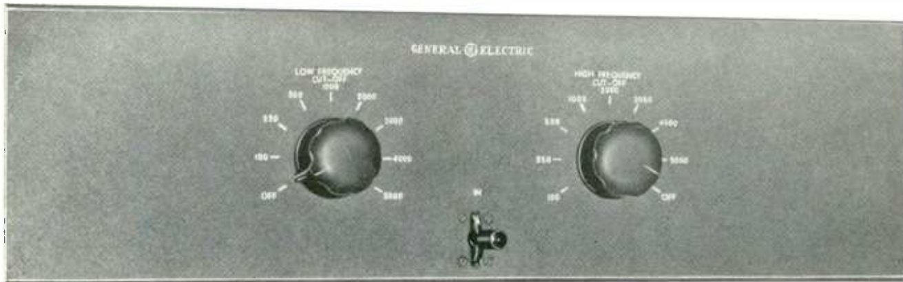
Sound effects filter panel, Type FA-18-A
