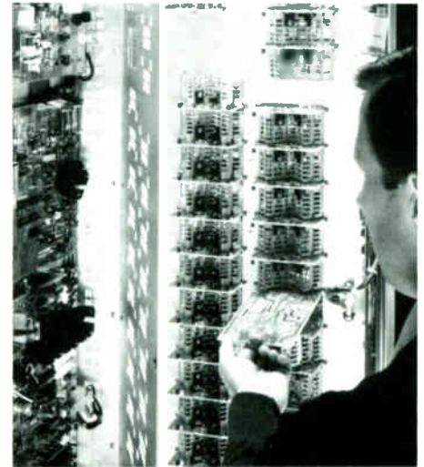
Modules are key to high efficiency, easy serviceability with the Harris DX-10.
