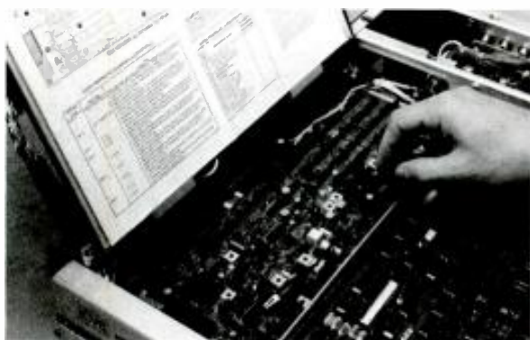
The unique "flat-pack" design of the CVS-517 makes all components easily accessible for fast, easy maintenance, testing and troubleshooting.
