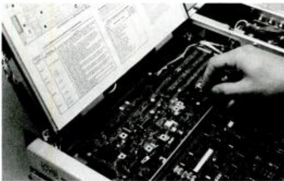
The unique "flat-pack" design of the CVS 516 makes all components easily accessible for fast, easy maintenance, testing and troubleshooting.
