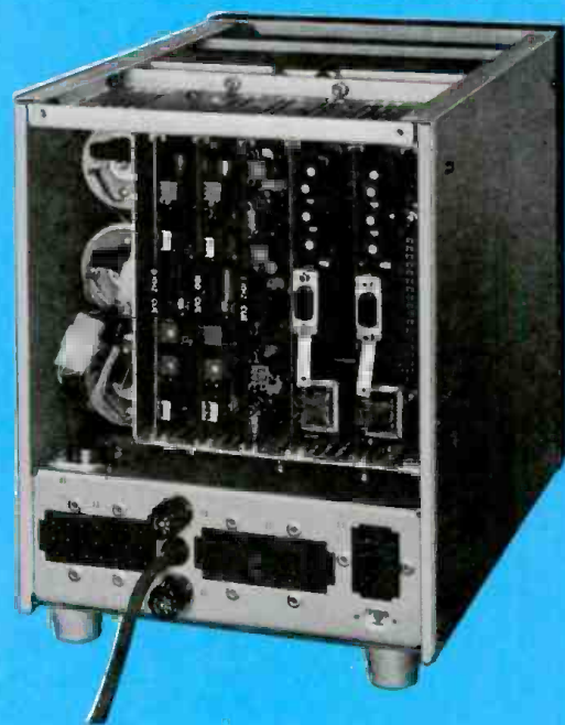
Two Criterion 90-3's may be mounted side by side in a standard rack to provide six playback units in a rack space that will hold only two regular size playbacks.
