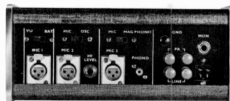
The rear panel shows the logical grouping of line terminations.
