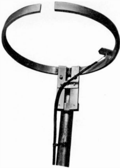
Left, FM-11 single ring omni-directional antenna with power gain of 0.8. Right, two bay FM-22 omni-directional antenna with gain of 1.6. These are broadband, easy to install antennas.
