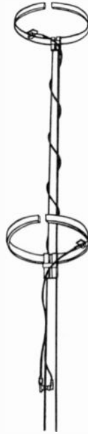
Left, FM-11 single ring omni-directional antenna with power gain of 0.8. Right, two bay FM-22 omni-directional antenna with gain of 1.6. These are broadband, easy to install antennas.
