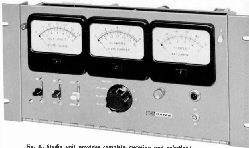
Fig. A. Studio unit provides complete metering and selection/operation of up to 23 control functions. Power supply is self-contained.
