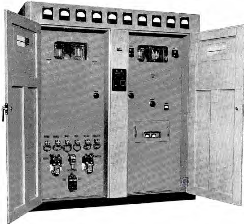
The front of the Gates BC-1F Transmitter has all controls behind a pair of firm free handling doors. As the "dead front" principle is apparent, no door interlocks are required. Note all relays and circuit breakers are at the finger tips.
