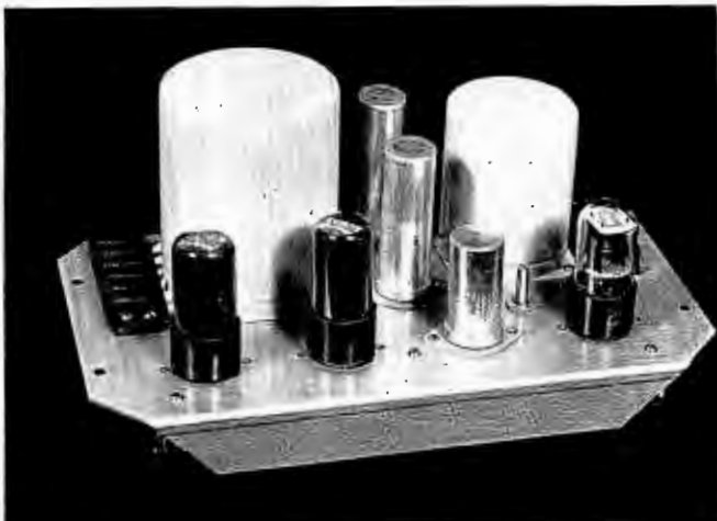
SA-96 two-watt monitoring amplifier illustrates another compact yet highly convenient way of obtaining the most from rack cabinet space. SA housings described on Page 154 are suggested.
