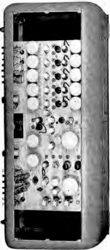
SA-40 console looking from top. All preamplifier tubes are shock mounted. Note heavy, sturdy construction of cabinet.
