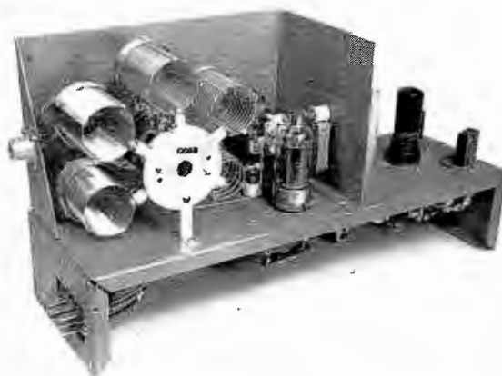
Rear view of oscillator-buffer unit illustrates turret coils for quick band change. Note plug-in oscillator which may be removed quickly for servicing.
