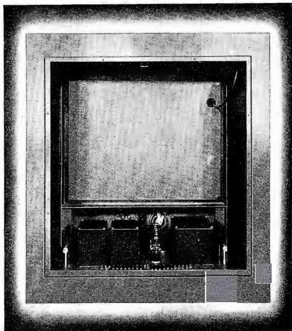
Rear view of the BF-E-10 transmitter shows the power supply in the bottom and the transmitter portion just above. The inside cover over the transmitter chassis is easily taken off by removing the four thumb screws in the corners and disconnecting the coaxial output feed line at the fitting on top of the transmitter.
