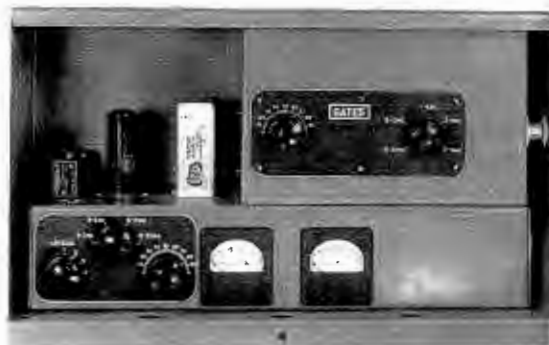
Front view of the oscillator-buffer section removed from transmitter. One of four crystals may be selected, and may be either temperature or non-temperature controlled.
