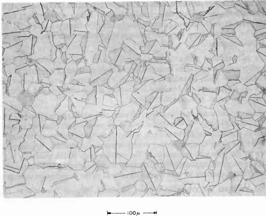
FIGURE 3.2: OPTICAL PHOTOMICROGRAPH OF A POLISHED AND ETCHED SECTION OF A GE-MOV® VARISTOR
