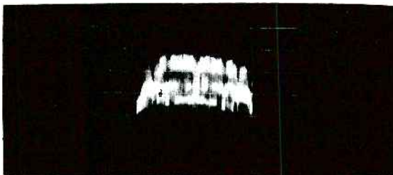
(e) Q5, Base, 0.25 volt P-P, H Rate (Typical Value Depends on Setting of Viewfinder Contrast Control)
