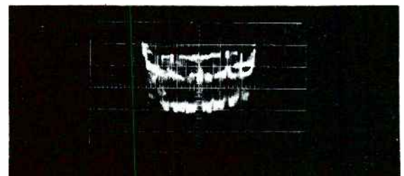
(f) Q5, Collector, 15.0 volts P-P, H Rate (Typical Value Depends on Setting of Viewfinder Contrast Control)
