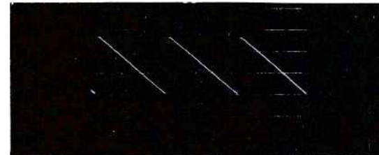
(f) P2-X, R Vertical Sweep Return, 15.0 volts P-P, V Rate, (Depends on Setting of W HEIGHT Control)
