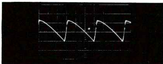
(e) P2-AA, W Vertical Sweep Return, 15.0 volts P-P, V Rate (Depends on Setting of W HEIGHT Control)
