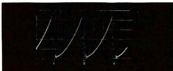
(c) Q17, Base, 0.80 volt P-P, H Rate (Depends on Setting of Master H Lin Control)
