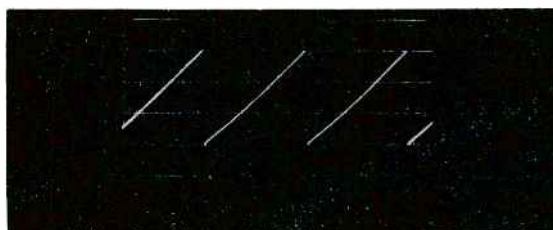
(b) Q1, Base, 1.5 volts P-P, H Rate
