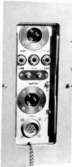
Fig. 5-33 Output end of BA-6-A Amplifier with cover plate removed
