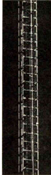
Side-mounted VHF-TV Transmitting Antenna
