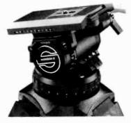
The Horizon II has a dynamic counterbalance system with 7 settings, which can be engaged with the 3 setting levers in order to compensate the tilt momentum resulting from the camera weight and the height of the center of gravity.
