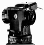
The Standard 7+7 has a counterbalance spring which is sufficient to balance an Arri 35 II/IIIC with a heavy zoom lens within the entire tilt range. Additionally, the counterbalance spring can be inserted in any chosen position within the tilting range when working with front heavy or tail heavy cameras, so the tilting range is not curtailed in any manner.
