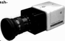
Standard C-mount lens compatibility = Video output NTSC composite video/RGB/sync • Imaging device 2/3" interline transfer CCD • Luminance S/N ratio >50dB (typically 53dB); chrominance S/N ratio >45dB (typically 48dB) • Scanning system 525 lines (12:1 interlace) • White balance preset and manual for video and flash-sync modes • Ambient gain control selectable 0dB, +6dB, +12dB • PC flash connector • Camera head mounting 1/4-20 UNC mount (standard video mount). Power requirement 12VDC 560mA = 3
