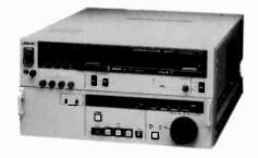
sumption • High speed picture search • Built-in time code reader and time base corrector • Built-in character generator and characters can be superimposed via Video Output 3 • RS-422 serial interface and 36-pin parallel interface • 59 lbs., 8 oz.; 5 rack units high
