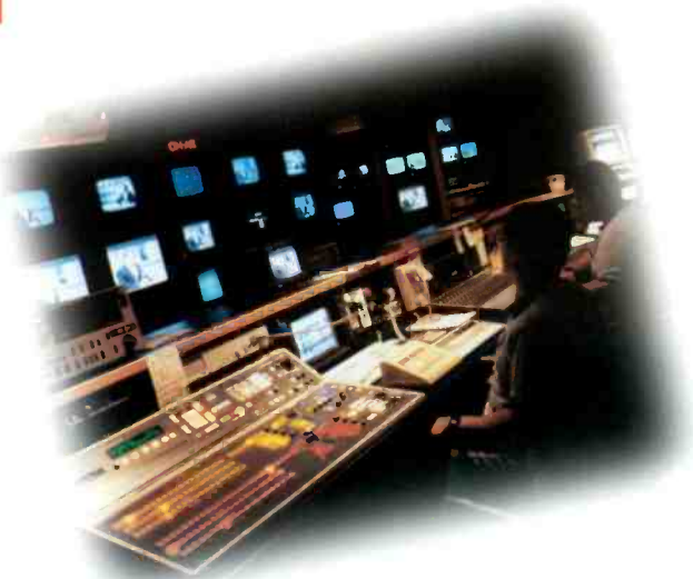
Three-channel automated master control system, News Channel 8 (Allnewsco) regional cable network, Springfield, Virginia
