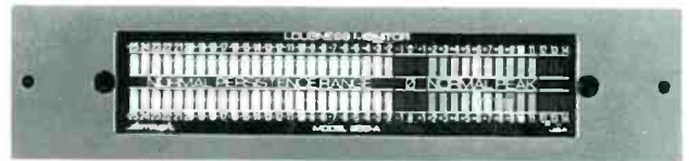
The two-channel AES/EBU meter
