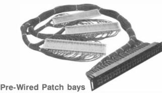
Complete selection of Bay types. One row, 24 to 26 jacks. Two rows, 24 to 26 jacks each and two row (48) bantam jacks. Complete selection of terminations available. Christmas tree, punch block, barrier blocks and Gentner flexiblock.
