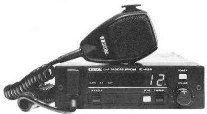
Now ICOM offers the fully synthesized IC-435 UHF mobile in both 2 and 12 channel versions. The IC-435 may be dash-mounted, or the front control panel may be unplugged and remote-mounted using the IC-R35 Remote Kit.
