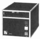
1. Delta I Reproducer: High speed recue and triple cue tones standard. Accepts "AA" cartridges. NAB 1975 equalization or CCIR. 110-240V; 50/60 Hz. 5.5/8"W  $\times 12$ "D  $\times 5.1/4$ "H.
