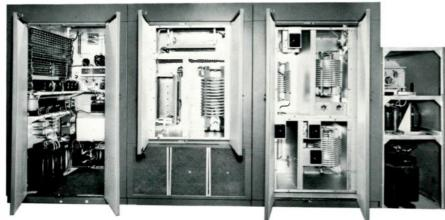
Continental's Type 317C is completely self-contained with the exception of the plate transformer which is in a separate self-contained enclosure. A 5 hp, 2,000 cfm blower housed inside the transmitter cabinet provides cooling and at a low noise level.
