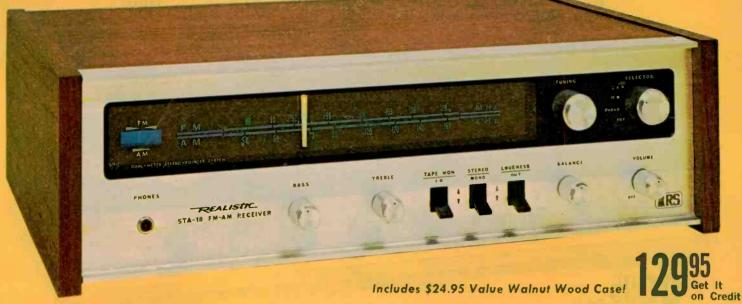
SPECIFICATIONS. Output at 8 Ohms: 25 watts  $\pm$  1 dB. 20 watts IHF, 14 watts rms. Response: 20-30,000 Hz  $\pm$  2 dB. Power Bandwidth: 30-20,000 Hz. Harmonic Distortion: Under 1%. Hum and Noise: -60 dB. Input Sensitivity: Phono, 2.5 mV; Output: 4-16 ohms. FM Sensitivity: 2.0  $\mu$ V. Separation: 40 dB. Signal-to-Noise: 67 dB.
