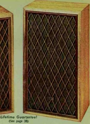
Nova-8. From the profundity of bass viol or tuba to the most acute lyrical highs, our best Nova speaker will compare with any and all of the finest! 12" acoustic-suspension woofer and 3 high-compliance tweeters. Deluxe capacitive-inductive crossover —the woofer cuts out at 800 Hz, 2 mid-size units cover 800-5000 Hz, tweeter covers 5000-20,000 Hz-4 elements in all. 8 ohms. 25x14x111/2"
