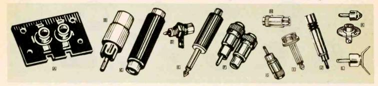
A DUAL PHONO JACK. For stereo changers, amplifiers, etc. Accepts RCA-type phono plugs. Provides quick, sure interconnection of audio equipment whose existing connectors do not mate. 274-332. Ship. wt. 3 oz.
