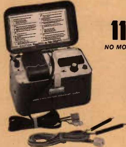
GM regulator drops into footproof fixture. When top is closed, regulator is heated to maximum under-the-hood temperature.
