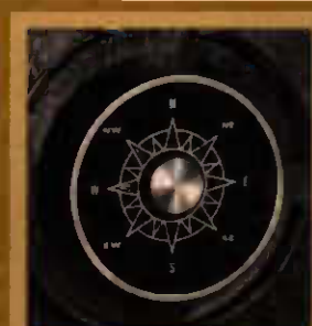
Wind direction is displayed with soft-orange lighted triangles within the "arrows."
