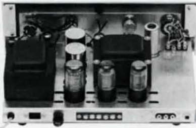
The inside of the new Heathkit AA-181 Amplifier shows the roomy arrangement for easy assembly and the sturdy components that guarantee long life.
