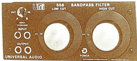
Universal Audio Variable Bandpass Filters. Models 555 (mono) and 556 (stereo)
